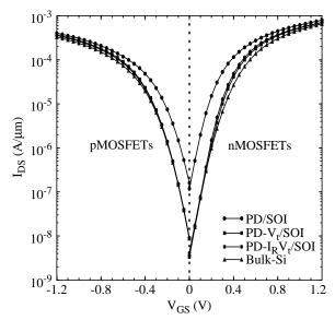
Fig. 4. UFPDB-predicted current-voltage characteristics of the  $L_{min}$ =50nm devices in the scaled  $L_{eff}$ =70nm PD/SOI and bulk-Si CMOS technologies; T = 27°C. The PD-V<sub>t</sub>/SOI and PD-I<sub>R</sub>V<sub>t</sub>/SOI curves are, respectively, for the FB V<sub>t</sub>-adjusted devices and hypothetical ones with higher (x10) I<sub>R</sub> in (2).
