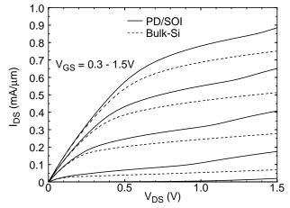
Fig. 2. UFPDB-predicted current-voltage characteristics of  $L_{eff}$ =70nm FB PD/SOI and bulk-Si nMOSFETs.
