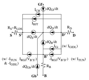
Fig. 1. Network representation of the UFPDB model.
